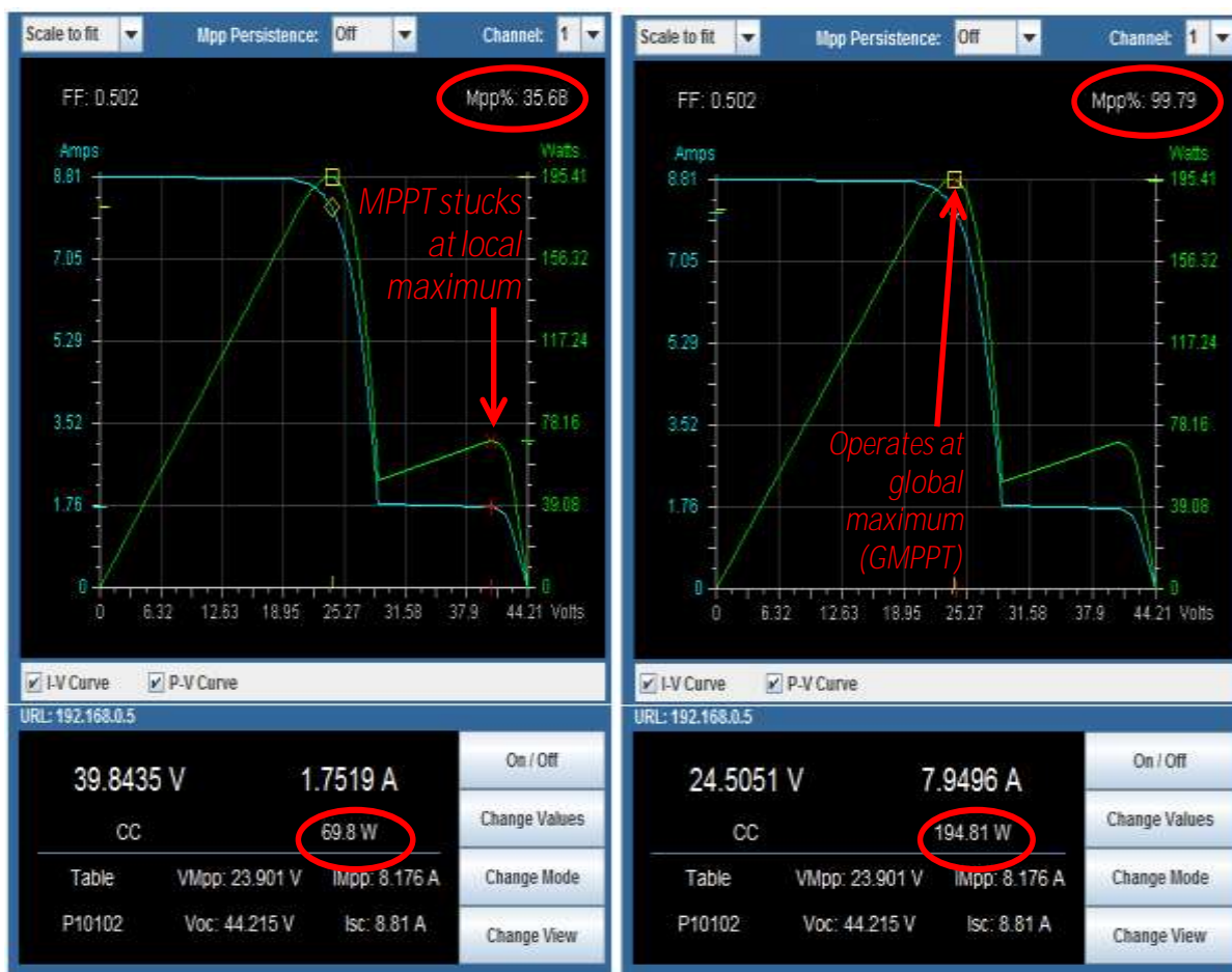
Fig. 7. Comparison of static MPPT efficiency and power captured from the 72-cell PV Module Trinasolar TSM-PD14-305 under the partial shading conditions. Premium competitor on the left, UBIK on the right.
