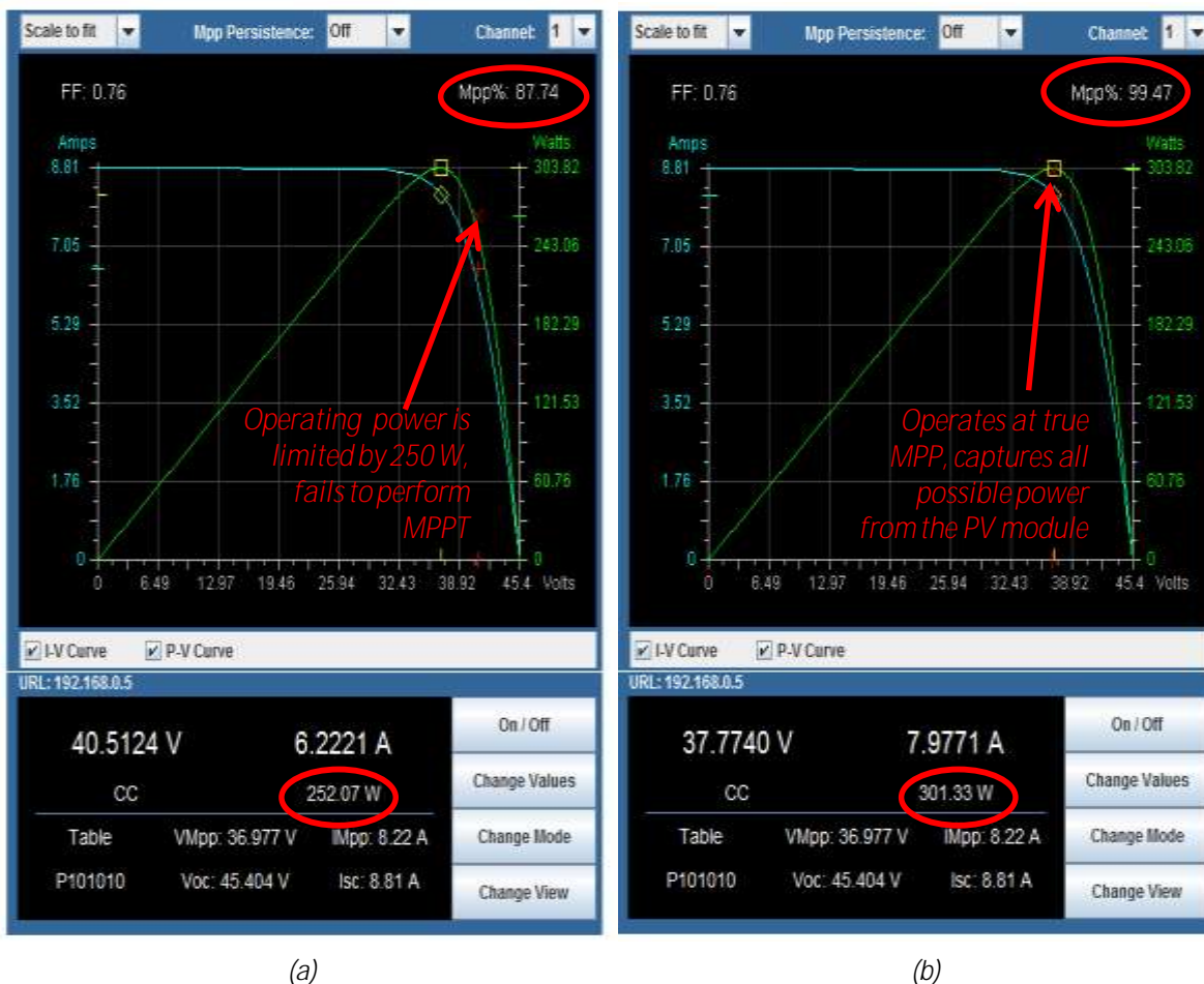
Fig. 6. Comparison of static MPPT efficiency and power captured from the 60-cell PV module Trinasolar TSM-PD14-305 under the partial shading conditions. Premium competitor on the left, UBIK on the right.
